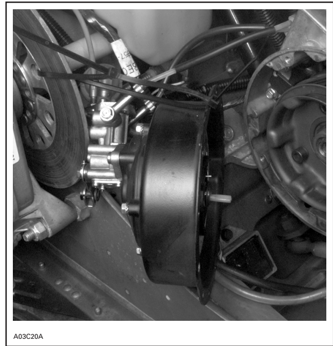
REWIND STARTER TEMPORARILY ATTACHED TO DISK BRAKE WITH LOCKING TIE
